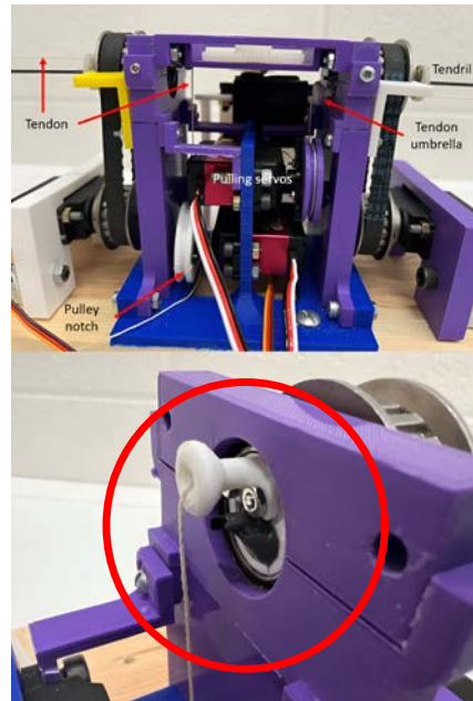
(Fig 3. Circled in red, the tendon routing in the old prototype does not allow for constant tension as the device rotates.)
