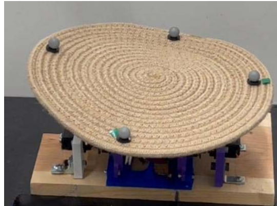
(Fig 2. The original robot surface prototype. Flexible surface shown with four markers attached for quantitative measurements. Actuation package below surface.)
