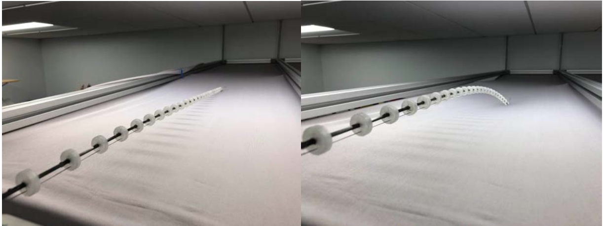
(Fig 15, 16. Arm at rest below fabric(Left), Arm at 140 degrees pulley rotation below fabric (Right))
